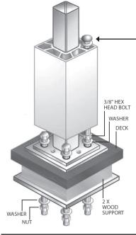
Once the set screw is removed, slide the Top Attachment Block up approximately 6" and align the bottom opening with the pre-drilled hole of the internal support post. Securely fasten the 1-1/4" set screw and you are ready for the 42" installation.
