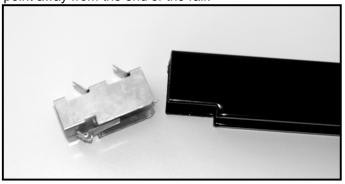
2. Slide the clip at a slight angle into the end of the rail using a glove or a plastic shipping clip to protect your thumb.
