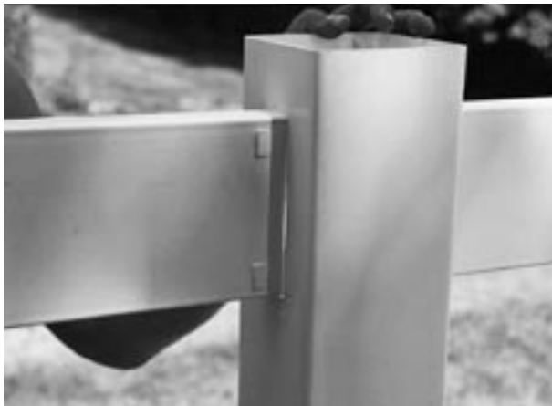
Country Estate rails utilize wedge locks that allow expansion without uncoupling, once pushed through the routed post opening.
