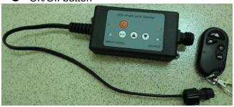
RF dimmer is a controller that can adjust light to the appropriate lighting brightness incrementally. Using the MODE button, click button to adjust from 100% - 70% - 35% - 5%. Pressing and holding the up/down arrow keys allows for micro adjustment between these increments. Pressing the MODE button again will bring the light back to previous increment. Press the  $\ensuremath{\mathbf{U}}$  button to turn lights on/off.
