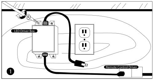
**POWER SOURCE:** Mount the LED Driver Box at least 18 inches above the ground near your outlet using screws. Do not plug it in. [ILLUS. 1]
