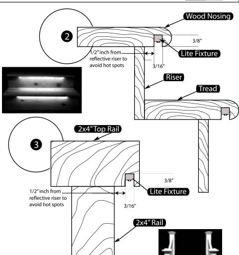
FOR STAIR INSTALLATION: [ILLUS. 2] using a table saw or router, cut a 3/16" wide x 3/8" deep channel the full length of the stair nosing. For best results, The LED Strip should be at least ½" from stair riser to avoid hot spots.
